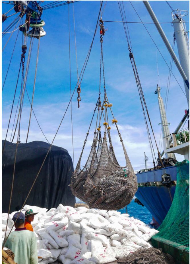
Photo 1: Transshipment Sling Structure
